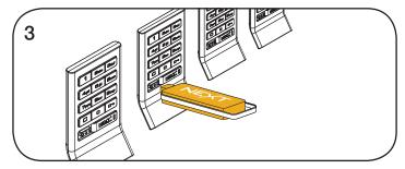
At each lock to be registered, insert the Programming Key. A two-tone beep will be heard and the LED will flash once to indicate successful registration.
