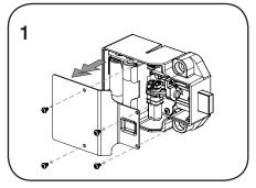
Remove the screws and the cover plate.
